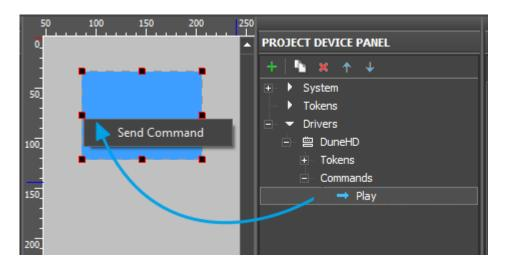
In the **Send Command** dialog window select the type of the event which will activate command sending to the device.
