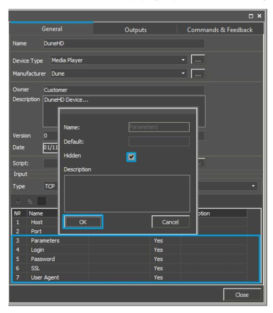
To add the command in the list of the created device go to the Commands & Feedback tab and use tools of the Editor base:
