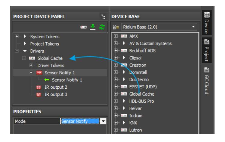
In order to use the channels of sensors states it is required to drag the Global Cache status channels from the Feedback tab to the project graphic items which should display the state of GC sensors. Numbering of the channels is based on the structure of Global Cache modules and outputs:
