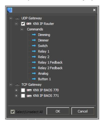
If you don't have an ETS project where you can import the required addresses from, you can create a gateway with datapoints manually. After the import or creating the device manually you can set up the connection and start working with the addresses.
