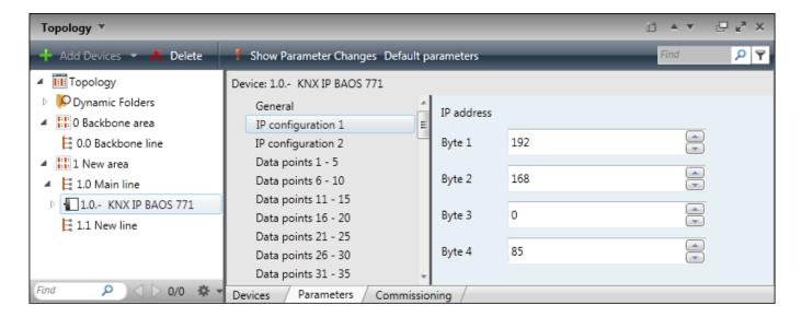
4. Intermediate addresses (datapoints) are activated and set up for connection with project group addresses in the "Data Points n...m" tabs. In datapoint settings indicate the address name and data type it will operate with. Select the same data type as the group address you want to relate to this datapoint:
