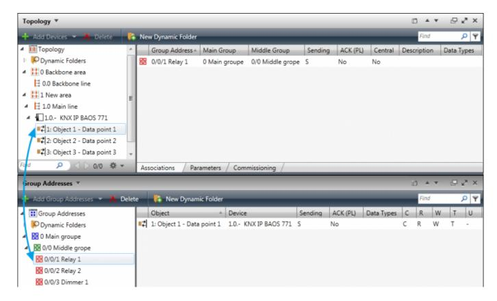
After all necessary relations are created save the project file in the ETS3 or ETS4 format (\*.pr3, \*.pr4, \*,pr5, \*.knxproj, \*.csv). Then the project can be imported in the GUI development environment of iRidium GUI Editor for fast setting up of communication with KNX.
