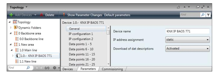
3. Go to the "IP Configuration 1" section in the list of KNX IP BAOS settings and indicate the IP-address of the KNX IP BAOS interface (the subnet mask and gateway address are indicated in the "IP Configuration 2" section by default):
