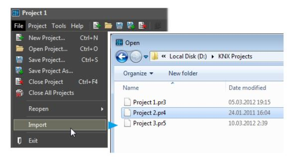
The tool of import from the ETS project forms the list of IP gateways and datapoints for them. You can select the gateways you need to add into your project from the list. As a result of the import you receive Project Device Tree containing imported interfaces and the list of addresses:
