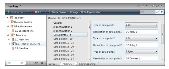
5. Relate the set up datapoint to the corresponding group address(es) by dragging it from the "Topology" window to the "Group Addresses" window:
