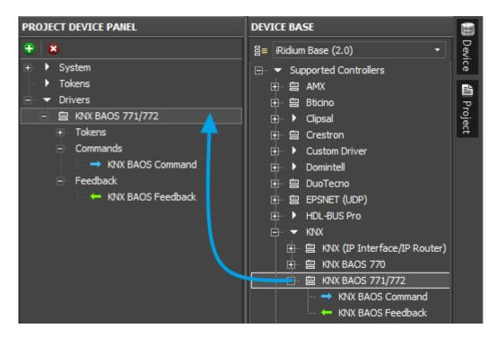
The commands to the bus and feedback channels are created and stored inside the gateway. Activation of command sending and displaying feedback data is performed by communication of commands and channels with graphical items of the interface.
