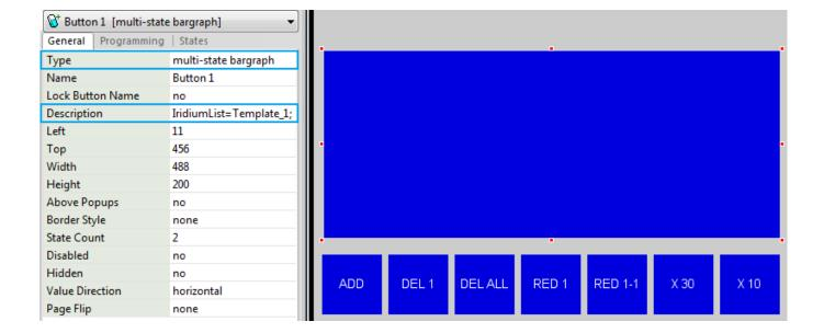
In the **Programming** tab of the list basis set up the way how information about pressing on the list components will be received. The information is sent to the AMX controller and the controller forms activation of the corresponding scenarios on its basis:
