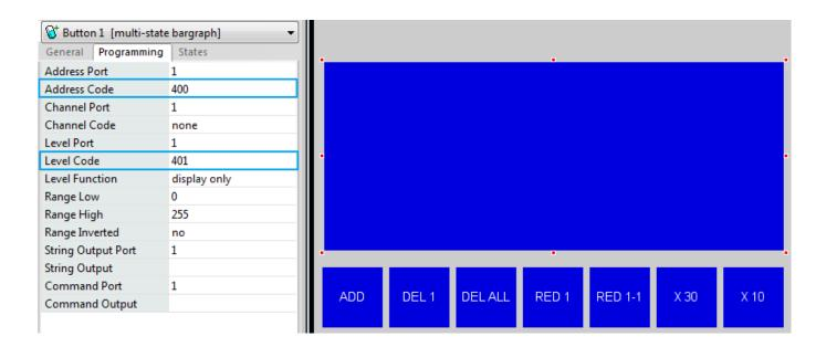
A standard Popup is always used as a template of the list component). The identifier of the first list component (ID of the first item) is indicated when forming the list with the help of the IRLB\_ADD command (see the list of commands). Sub-items of each list component are standard buttons or other graphic items.
