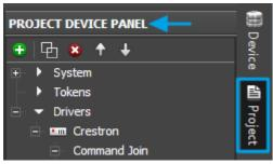
**Project Device Panel** is used for creating the tree of GUI devices. You can add devices selected in *Device Base* or your own base by the Drag&Drop method here. All controlled devices and GUI channels are created and set in this tree (the *Properties* window in the lower part of *Project Device Panel*).
