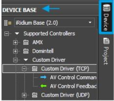
The **Device Base** panel opened by clicking the button on the right side panel of GUI Editor) contains the base of equipment and protocols supported by iRidium.
