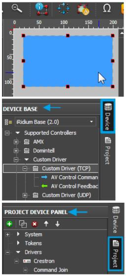
**Workspace** is used for positioning graphic items on GUI pages and popups. Here you can create and select an object which properties are set in the *Object Properties* window. Editor Workspace can be scaled. The objects of Workspace can be created with the help of the Draw Item tool and can be located with the*Select* tool.
