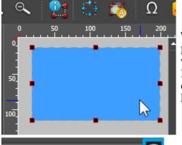
**Workspace** is used for positioning graphic items on GUI pages and popups. Here you can create and select an object which properties are set in the *Object Properties* window. Editor Workspace can be scaled. The objects of Workspace can be created with the help of the Draw Item tool and can be located with the *Select* tool.
