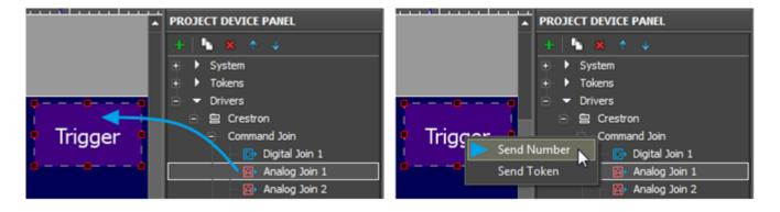
To send values to the controller select **Send Number** – send a number in the decimal format. After selecting Send Number the window (input field) is opened where you are required to write the value sent to the join at pressing on the graphic item:
