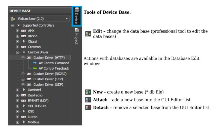
In Device Base Editor you can create custom drivers for controlling equipment, select the device type, create commands, feedback channels and script modules for data processing.
