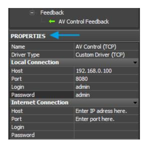
Object properties selected in the Project Device Panel tree (settings for connection with equipment – an IP-address, port, specific equipment properties; properties of commands and status channels) are displayed in this window.
