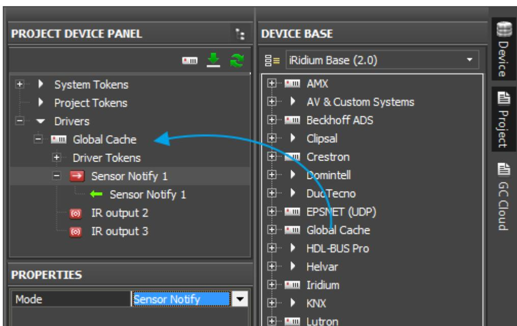
Global Cache sensors are discrete, i.e. they give values 1 or 0 (on/off). So the sensor status can be output as a text (1 - the contact is closed, the sensor was activated; 0 - the contact is opened) or by changing the state of the graphic item from inactive (0, State 1) to active (1, State 2). To make the status channel affect the state of the graphic item drag the channel to the item and indicate the property "In Value" (affect the item status):
