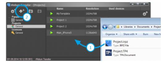
Add the panels (iOS/Windows/Android/OS X) you want to upload the module on and licenses (Device License **Pro** for AV & Custom Systems). In order to do that use instructions in the following section
