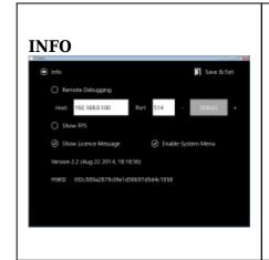
**Remote Debugging**. It sends the log of i2 Control V2.2 work to the remote PC with the installed Syslog server. The server address and logging depth are set up.
