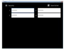
**Password 1 - Password 4** - <u>passwords</u> for accessing project pages. They can be changed for the project version uploaded on the panel. When using passwords it is recommended to disable the option of entering the menu "on hold" in the tab Info (Enable System Menu > Off)
