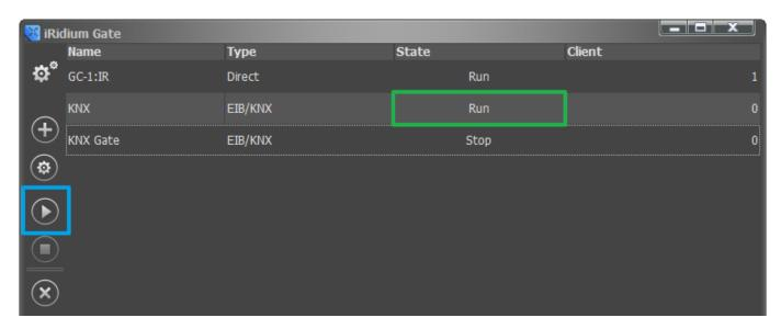
The number in the "Client" column shows the list of control panels (iRidium Apps) which are connected to the gateway at the moment.
